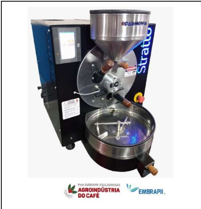
Figure 1: Machado Campus investment in research for portable energy-efficient electric roaster that replaces gas-fired roasters.
