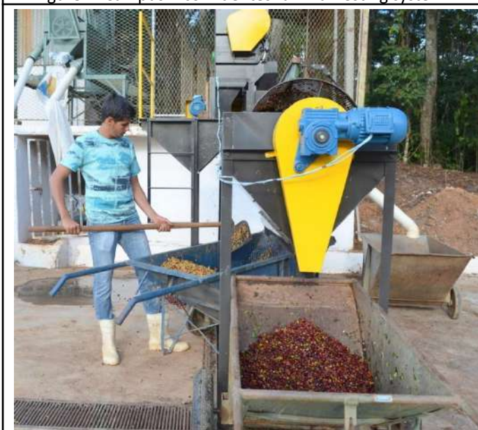
Figure 3: Campus Machado first invention patent, a water-free coffee peeler machine.
