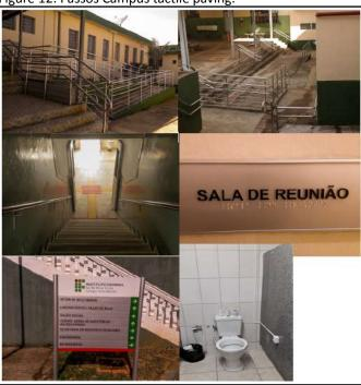
Figure 14: Inconfidentes Campus tactile paving, ramp, handrails, Braille nameplates and bathroom for people with disabilities.
